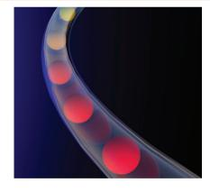
The controlled synthesis of semiconducting polymers in droplet-based microreactors is described. Using poly(3-hexylthiophene) (P3HT) as a test polymer, a product of controllable molecular weight and high regioregularity (>98%) is obtained at rates of up to 60 g/day. The droplet-synthesized P3HT yields power conversion efficiencies of 4% when combined with [6,6]-phenyl-C61-butyric acid methyl ester (PCBM) in bulk heteroiunction solar cells.
