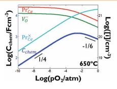
Chemical capacitance is demonstrated to reliably measure the oxygen content of an oxide thin film. A key step in this analysis, the derivation of absolute oxygen vacancy concentration, is achieved using defect equilibria based power laws (see figure). Thermodynamic constants defining defect generation are extracted from the data and general agreement with bulk values is found, despite evidence to the contrary in the literature.
