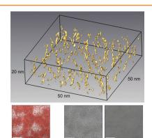
Organic-inorganic composites fabricated via co-evaporation of two materials reveal a filamentous nanostructure with filaments preferentially oriented perpendicular to the substrate plane. This growth process can be controlled by changing the substrate temperature so that for films evaporated on cooled substrates no filament growth can be detected.
