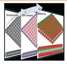
**2D, single-layer nanostructures** of transition metal carbides and nitrides, so-called MXene, here  $M_2C$  (M=Sc, Ti, V, Cr, Zr, Nb, Ta) and  $M_2N$  (M=Ti, Cr, Zr), which are chemically functionalized by F, OH, and O groups, are shown to have potential applications in optoelectronic, spintronic, and thermoelectric nanodevices based on first-principles calculations.
